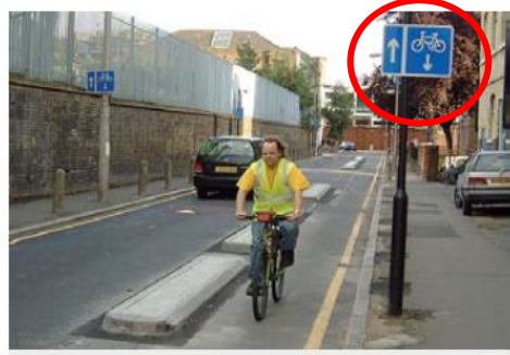
Contraflow with island separators, and showing the diagram 960.1 sign
