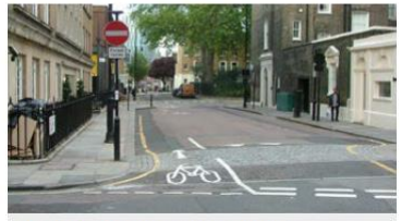
No entry with 'except cycles' plates, and raised table entry
