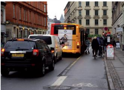
Bus boarder: a type of bus stop where passengers board and alight across a cycle lane
